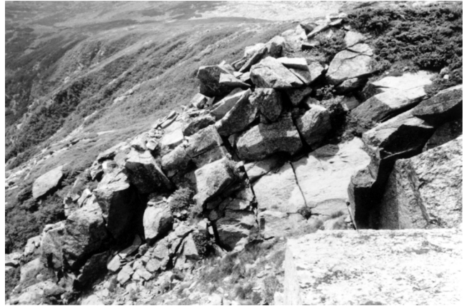
FIGURE 4. An example of block toppling that exhibits a "domino effect" on the west side of Connection Gully, the couloir above Site 2.
