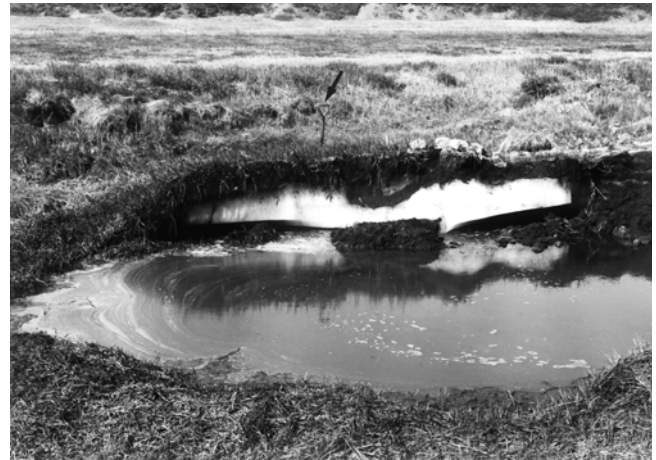
FIGURE 31. The intrusive ice was formed by the rupture of ice-bonded permafrost and the injection of sub-permafrost water into the active layer during the autumn freeze-back of 1985. The scale is given by the handle of a 1 m long shovel, marked with an arrow. Water quality analyses for the 5 ice samples, collected at 10 cm intervals, are given in Table IV.
