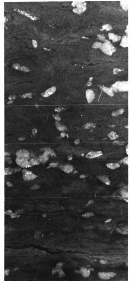
Figure 3 Red dolomitic mudstones with anhydrite pseudomorphs after gypsum crystals, Watrous Formation, Saskatchewan. Probable playa flat deposit. Core 10 cm across.
