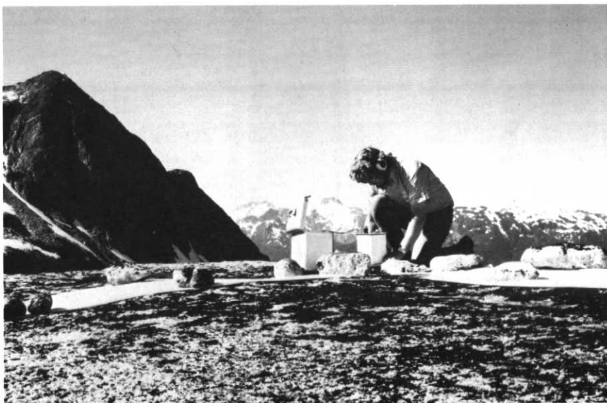
Figure 5 Today, La Coste and Romberg model G gravity meters are used for all land surveys made by the Earth Physics Branch.
