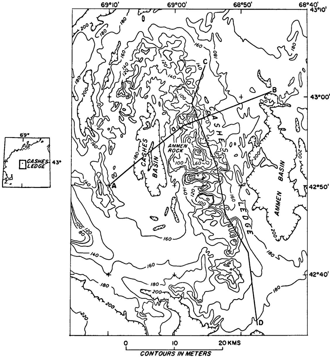
**Figure 1.** Bathymetric chart of Cashes Ledge. Contours are based on U.S. Coast and Geodetic Survey hydrographic surveys H-6564 and H-6566. Lines marked AB, CD and ab show the locations of the seismic and bottom profiles, shown in Figure 2 and Figure 3.
