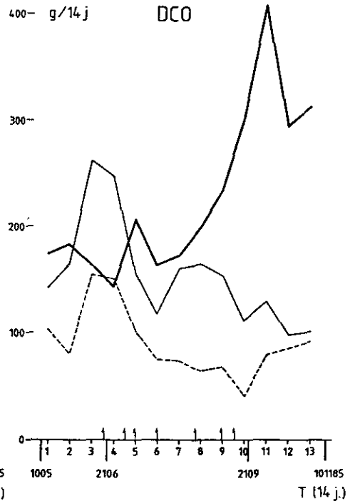
Figure 3 Flux de la DCO totale en C2 et C4 C.O.D. flux in C2 and C4
