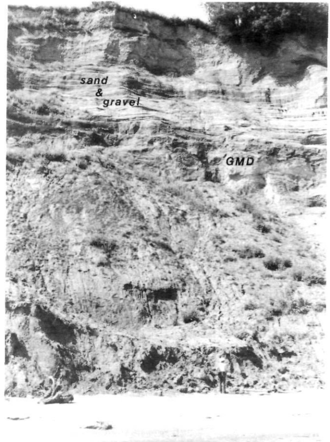
FIGURE 12. Possession glaciomarine drift (GMD) overlying Possession till at Point Wilson. The glaciomarine drift is overlain by Vashon advance outwash (sand and gravel).
