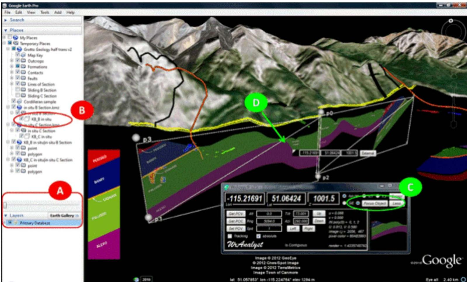
Cross sections *in situ*, meaning that the subterranean structures are shown in their original locations. In this case, the Google Earth primary database is removed from view and a “cut away” surface tile is inserted in its place as a <GroundOverlay> with terrain exaggeration set to one. The “cut away” can be achieved automatically using the line (yellow) which indicates the location of these cross sections along the surface.
