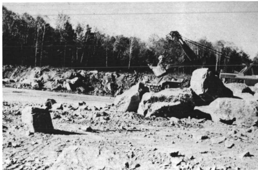
Figure 1 Extremely stony till rich in large limestone boulders at the Marmora iron ore mine, southern Ontario. (Photo A. Dreimanis).
