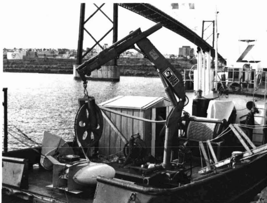
Figure 1 The DTS system aboard Survey Venture showing the winch, cable, crane, sheave block and towed body. The V-fin towed body in the background is associated with a Kelvin Hughes 26B echo sounder.
