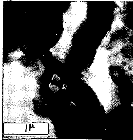
Figure 4 - High voltage transmission electron micrograph of flocculated grundite illite impregnated with polyethylene glycol. Flocculated in salt water ( \text{Na Cl } 1\text{ gm/l.} ) x 28000.
